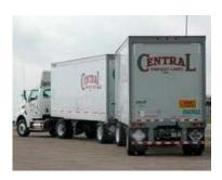
Waco, Texas-based Central Freight Lines has added 100 compressed natural gas (CNG) tractors to its fleet of more than 1,600. Central is a less-than-truckload general commodities carriers. The 2014 Freightliner M2 112 CNG tractors are powered by the Cummins Westport ISL G natural gas engine.
