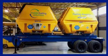
The Virtual Pipeline system, designed by Galileo Technologies and distributed by Verdek LLC to transport natural gas by road where there are no pipelines, will be used as a mobile CNG station.
