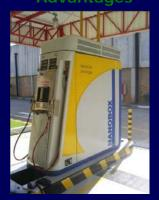
The Nanobox® has no special installation requirements. A simple base-plate gives sufficient support. Because of the low power required and incorporated electric panel, no special electrical installation, nor power transformers, nor external panels are required.
